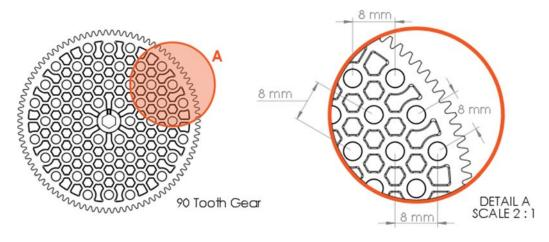
Figure 26: Motion Component Bolt Pattern Detail
