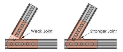
Figure 13: Extrusion with Beveled Joint
