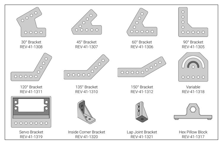
The REV Robotics 15mm building system uses plastic nylon (PA66) molded pillow blocks. The bearing pillow block can be used with the long through-bore or end cap bearings to provide a low friction shaft support. The hex pillow block directly interfaces with a 5mm shaft which can be used to drive a light duty arm or as a dead axle support.
