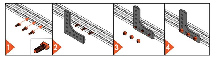
Figure 44: Drop-in Bolt Assembly Method
