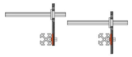
Figure 5: Shaft Offset Using an Indexable Bracket
