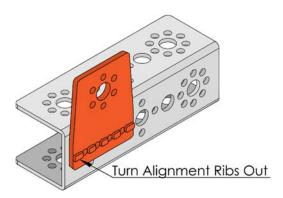
Figure 58: REV Robotics Plastic Bracket on Tetrix Channel with Alignment Ribs Facing Out
