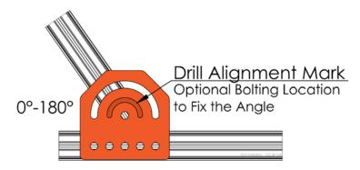
Figure 3: Adjustable Angle Bracket Example
