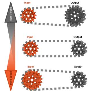
Figure 31: Using Sprockets to Increase Speed or Torque
