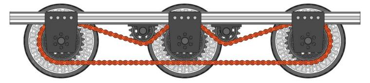
Figure 50: Example Sprocket and Chain Drive Train
