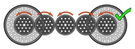
Figure 48: Correct All Gear Drivetrain
