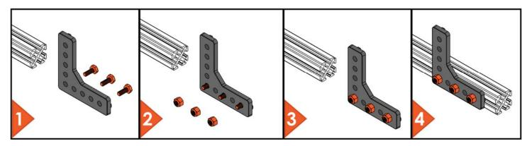
Figure 41: Preassembled Bracket Installation Method
