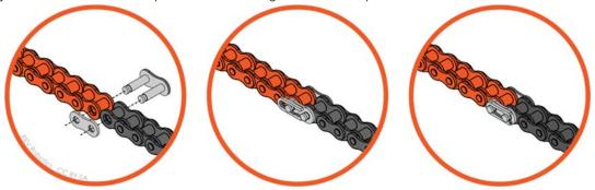
Figure 38: Master Link Assembly on Chain
