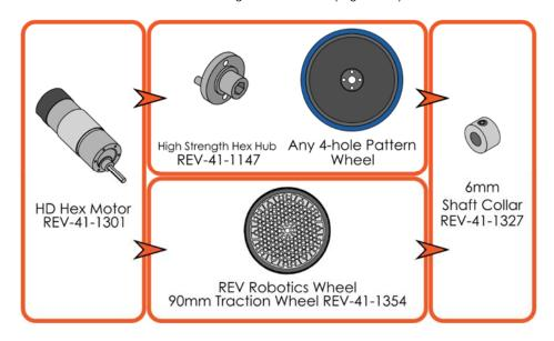
Figure 55: Direct Driven Wheel Using Hex
