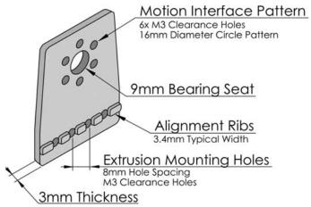
Figure 2: Motion Bracket Feature Details
