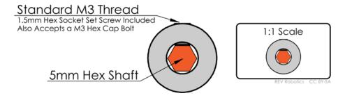
Figure 20: Shaft Collar Tightened on a Hex Shaft
