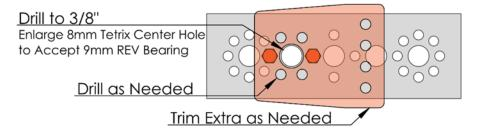
Figure 61: Using REV Robotics Bearings with the Tetrix Hole Pattern
