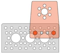
Figure 62: Motion Bracket Mounted to Actobotics Channel
