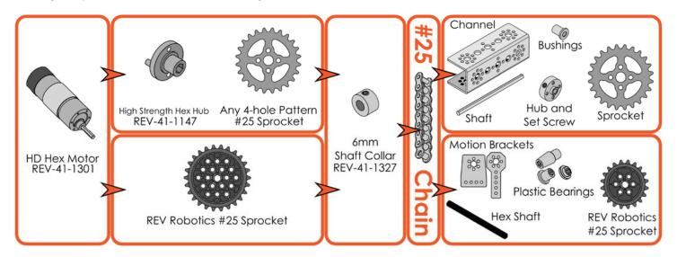
Figure 56: Sprocket and Chain Drive with Hex
