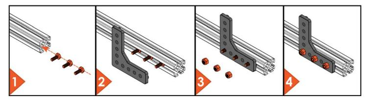
Figure 42: Bolt-first Assembly Method
