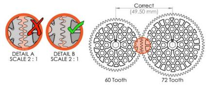
Figure 40: Gear Spacing Example
