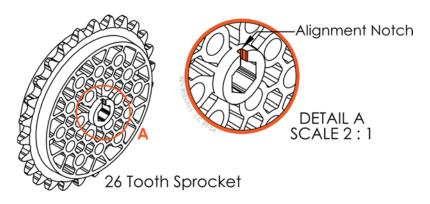
Figure 27: Shaft Alignment Notch Detail
