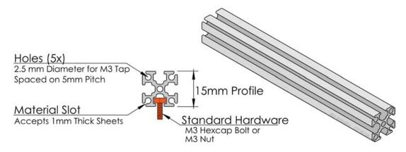
Figure 1: Extrusion and Cross-Section Details
