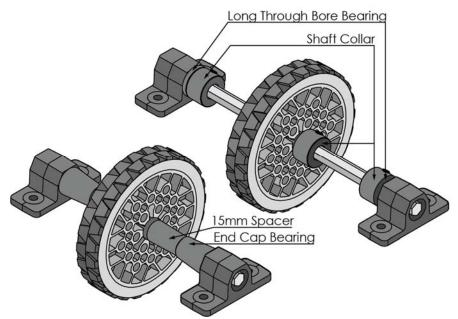
Figure 22: Shaft Collar and Spacer Side by Side
