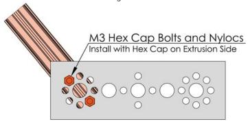
Figure 60: Mounting 15mm Extrusion to Tetrix Channel
