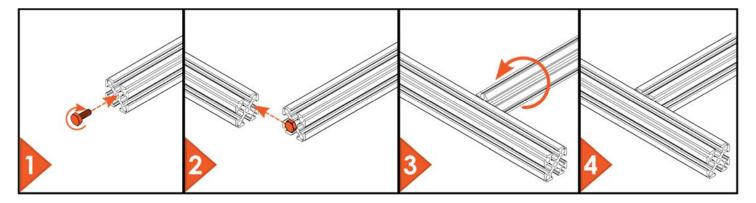
Figure 45: Extrusion to Extrusion Quick Joint
