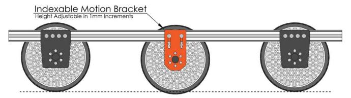
Figure 46: Drop Center Wheel Using an Indexable Bracket
