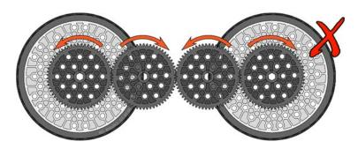
Figure 49: Incorrect All Gear Drivetrain
