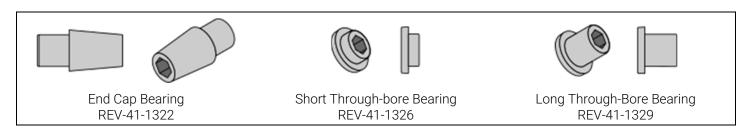
**End cap bearings** are closed on one end, so when these bearings are placed on both ends of a shaft and fit into motion brackets the shaft is free to rotate but is fully constrained laterally (sideways).
