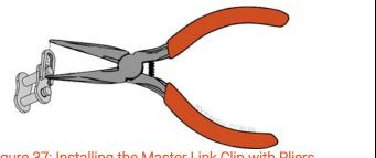
Figure 37: Installing the Master Link Clip with Pliers
