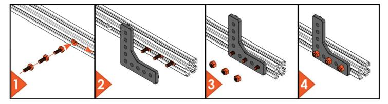
Figure 43: Access-hole Assembly Method
