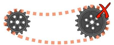
Figure 32: Incorrectly Spaced Sprockets (Chain too Loose)
