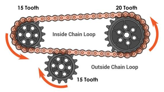
Figure 51: Single Stage Reduction (15:20) with Idler
