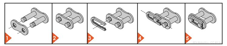
Figure 36: Master Link Detailed Assembly for Reference
